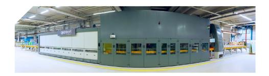
is subject to exacting quality requirements, for example with respect to glass thickness and curved surfaces. The Glaston-developed GlastonAir™, in which glass is transported and heated on a bed of air, meets these requirements very well. With GlastonAir™, it is possible to process 2.0 mm thick fully-tempered glass and 1.6 mm thick heat-strengthened glass that is extremely smooth and optically the best possible quality.
