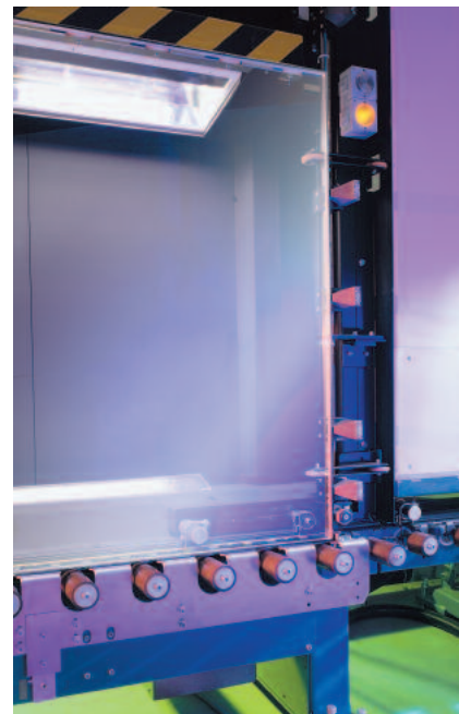
Automatic adjustment of frame positioning girder according to present glass thickness
