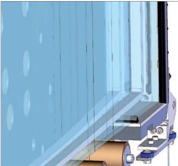
Filling the triple insulating glass unit with inert gas
